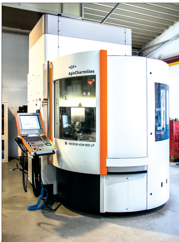
HSC Fräsmaschine Mikron SM800LP.
